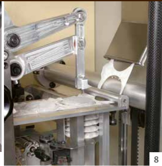
Electronical pod counting and stacking
