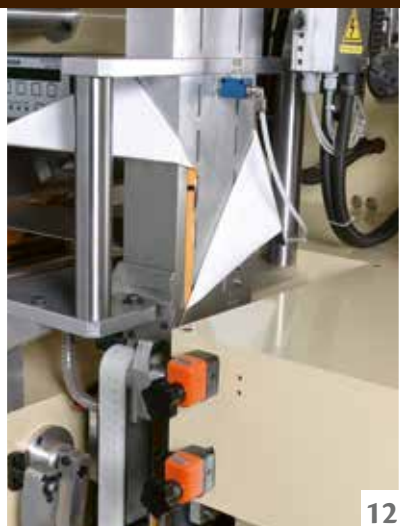
Integrated heatsealable pack forming
