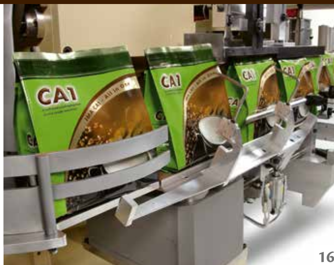
Top flap folding and pack exit
