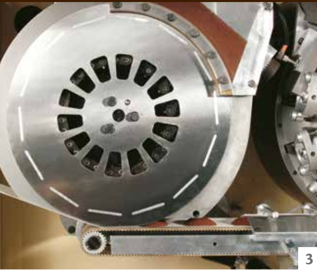
Volumetric doser with patented product compacting system
