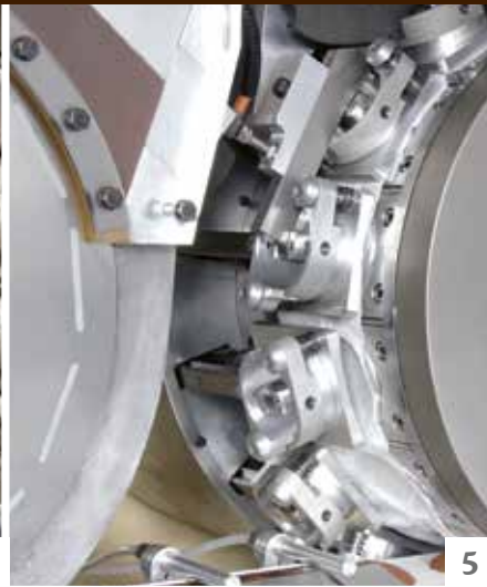
Mechanical filter paper pocket pre-forming wheel
