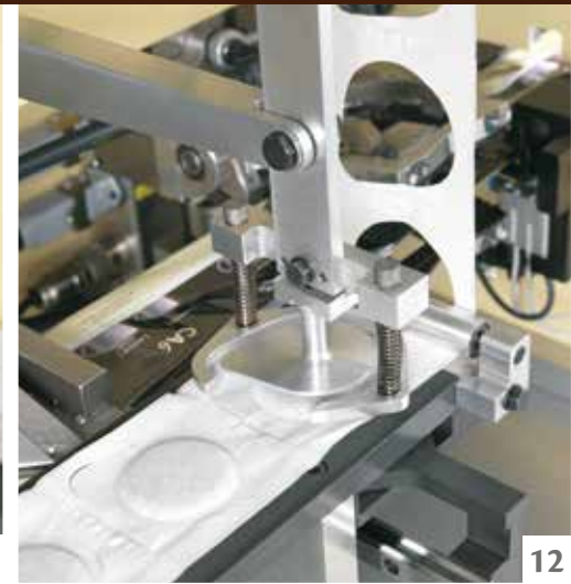
Pod ejection and insertion into outer envelope
