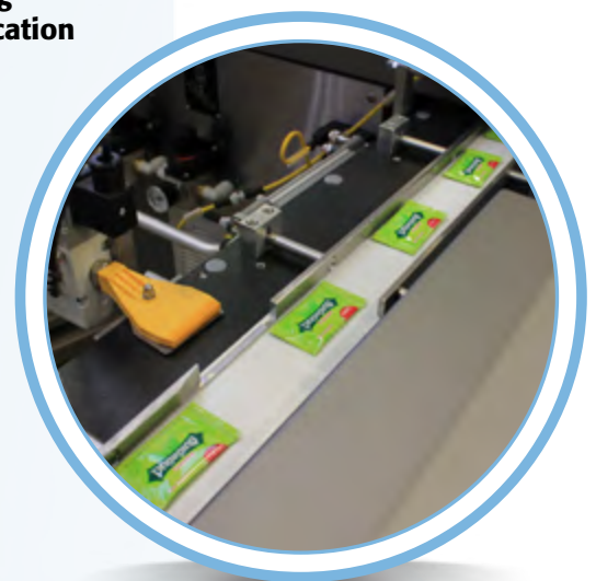
Outfeed exit belt
