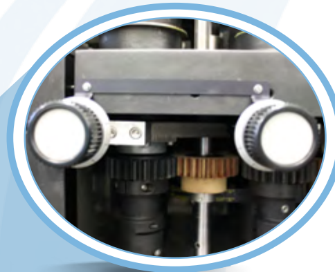
Longitudinal sealing rollers with auto-lubrification gears system
