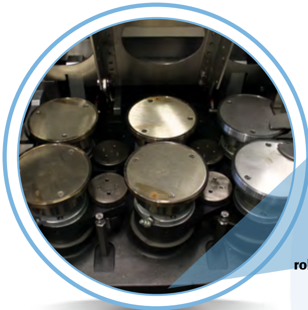
Cross sealing jaws, CNC machined from solid extrusion
