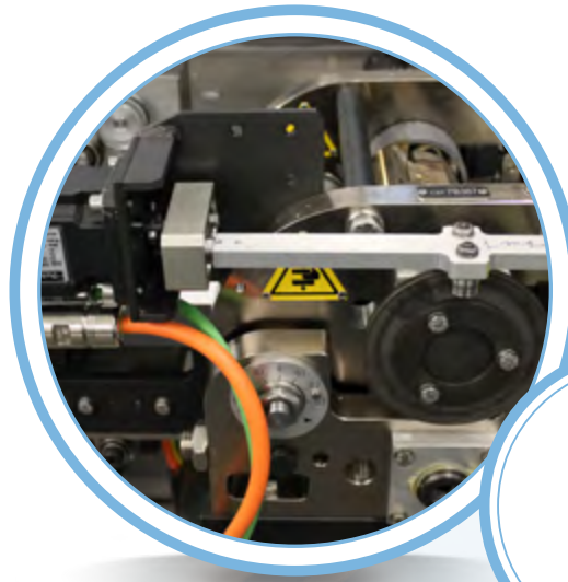
Cross sealing jaws, special execution for chain packs
