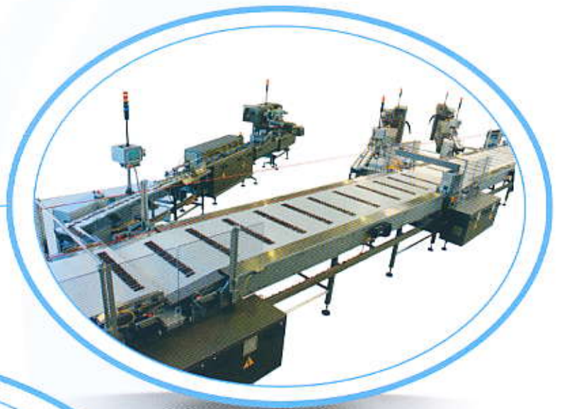
Multiple wrapping line - SMART distribution systems for enrobed cakes
