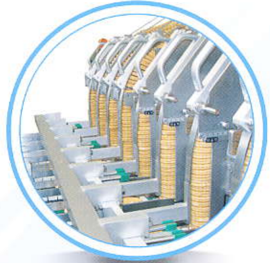
Single biscuit collection from gravity feeders
