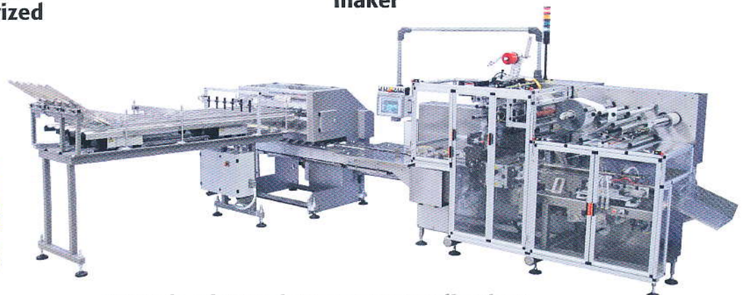
Example of Eurosicma Group application: Wrapper Eurofold Model combined with Portion Feeder APFV
