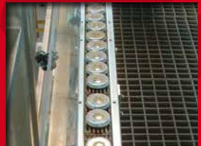
The capping machine model MS 250 has been designed to satisfy the medium speed productions up to 300 cpm. Thanks to the reliability and to the quick and easy format change operations and to the high level of hygiene and vacuum standards reached, the machine perfectly fits in the market of beverages and preserves.
