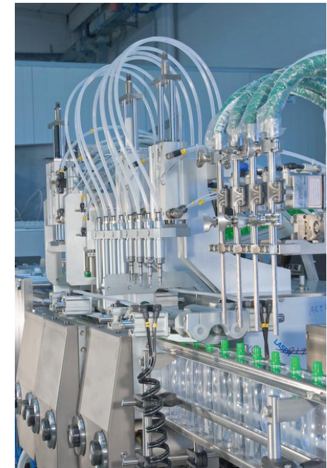
THE FORMING AND THE FILLING STATIONS
